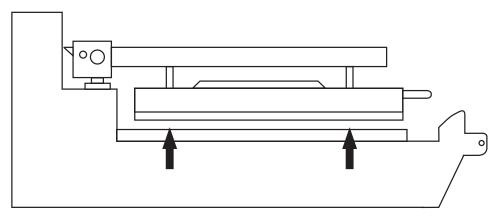
Insert gap tool directly below platen adjusters.
